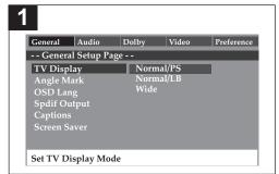
**NORMAL/PS:** Pan Scan. Select when the unit is connected to a conventional TV. Video material formatted in the Pan Scan style is played back in that style (the left and right edges are cut off).
